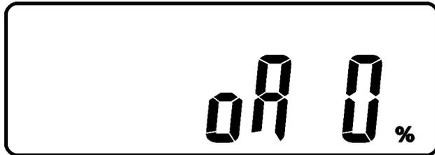
\* It shows Output Voltage Adjustment % from 0% to 3% or -0% to -3%.
