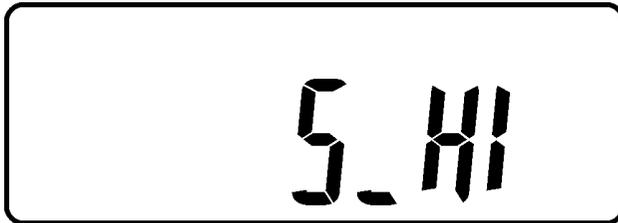
\* It shows bypass voltage is adjusted to wider one.
