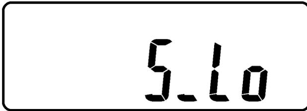
\* It shows Bypass Voltage is adjusted to narrow one.
