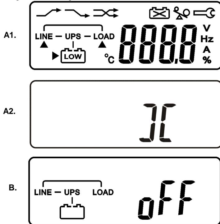
3.5.1.5 Then, the UPS is on Bypass Mode now and it will proceed self-test automatically. If there is no abnormal message occurred, it means the pre-startup of the UPS is successful and the charger starts to charge the batteries.
