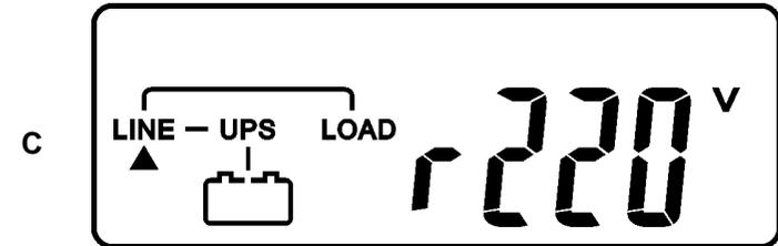
3.5.1.8 Then, the UPS is under self-test mode again, the LCD display will illustrate from drawing C to drawing D and remain approx. 4 seconds under battery mode, then illustrate from drawing E1 to drawing F if the self-test is successful.
